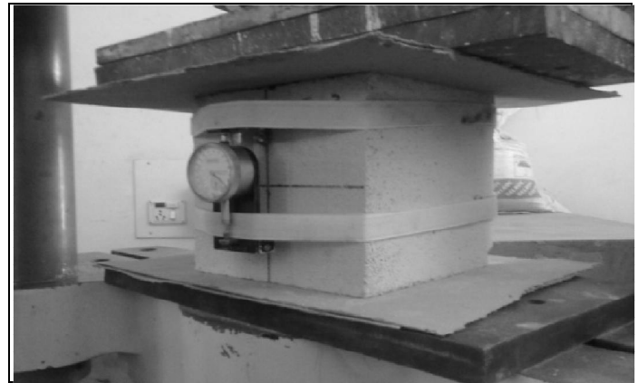
Plate 1: Stress-strain measurement under compressive load
