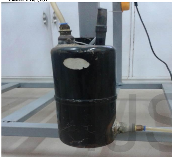
Fig-6: Drying unit.
