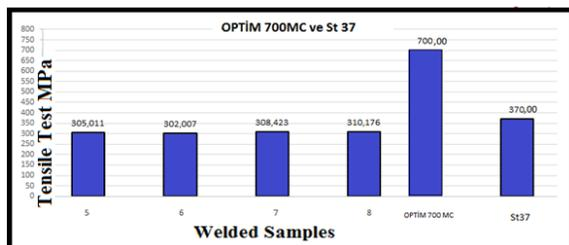
Fig. 5. Tensile graphs of the samples
