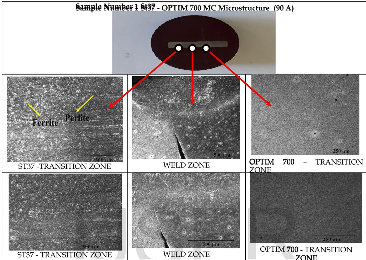
Fig. 3. Sample Number 1 St37 - OPTIM 700 MC microstructure (90 A)
