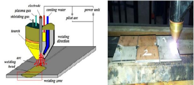
Fig.1. Schematic view of PTA welding and Image of PTA welding process [15].
