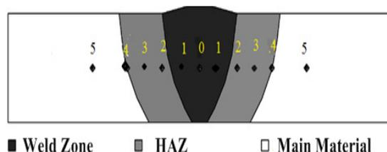
Fig. 6. Schematic view of micro hardness measurement points.
