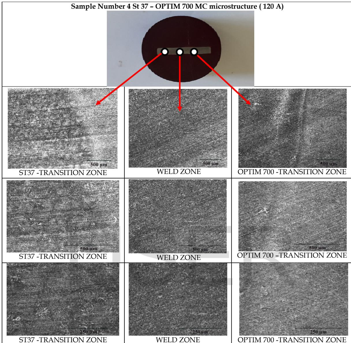
Fig. 4. Sample Number 4 St37 - OPTIM 700 MC microstructure (120 A)
