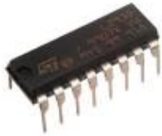
Fig: 3 L293D H-bridge (IC)
