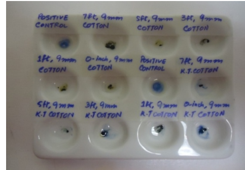
Figure 1: DPA test performed on cotton and K.T Cotton with 9mm Pistol
