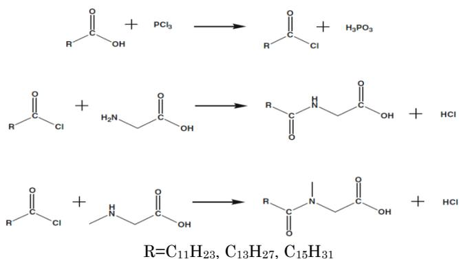
Fig. 1 Synthesis route to glycine and sarcosinebased surfactants
