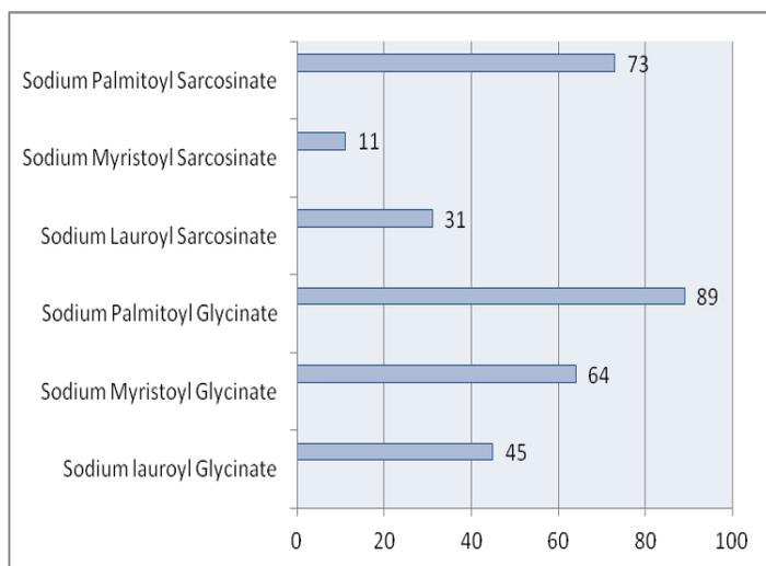
Fig. 7 Wetting time of glycine and sarcosine based surfactants
