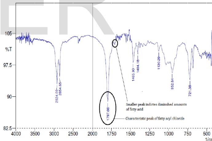
Fig 2 FT-IR spectra of Lauroyl chloride
