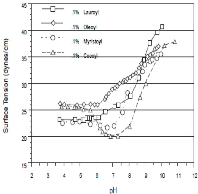
Fig 4. Surface activity of N-acyl sarcosinate with respect to pH changes [24]
