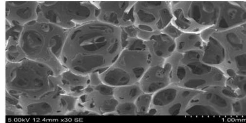
Fig. 4c 1.4% Crumb rubber in PU foam
