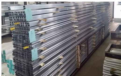
Fig. 6 – Over stacking of materials in the rack.
