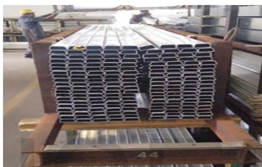
Fig. 7 – Properly stacked materials in the rack
