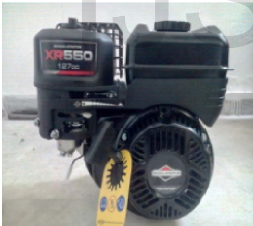
Fig. 4 “BRIGGS AND STRATTON” engine of 127cc with 3.5 HP
