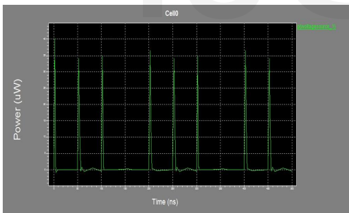
Fig.28 Waveform for Power of 1:1 Ratio CMOS Inverter
