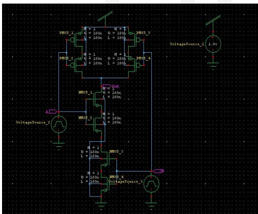
Fig.44 Stacking CMOS NAND Gate
