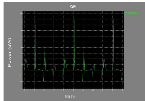
Fig.49 Waveform for Power of Adiabatic CMOS Inverter
