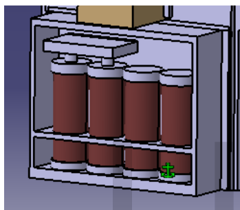
Fig. 10. The CO 2 storage.
