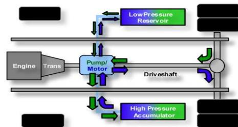
Fig 3: Hydraulic assisted RBS
