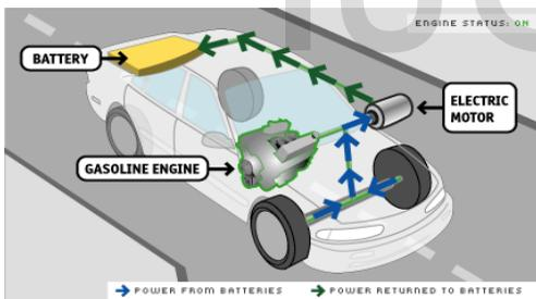
Fig 1: Motor-Generator RBS
