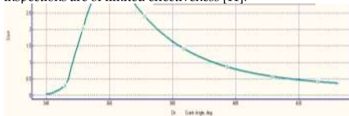
(a) Plot of Soot against crank angle @ 1500 rpm
