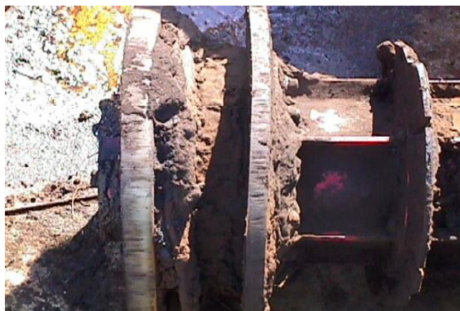
Fig.9. Cleaning paraffines by pig
