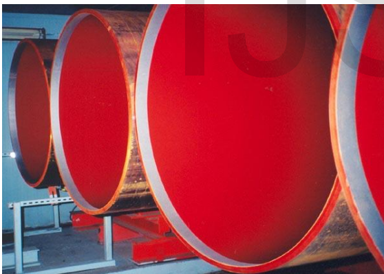
Fig. 6. Reducing paraffine by epoxy layers
