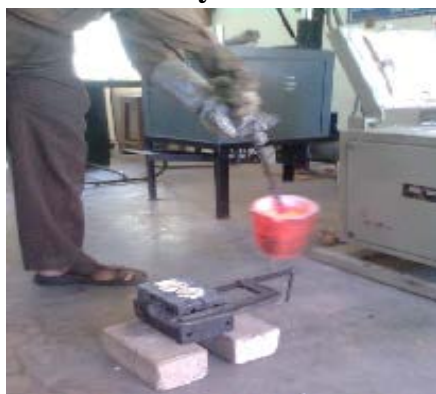
Figure 2.1 Stir casting furnace with raw materials set up
