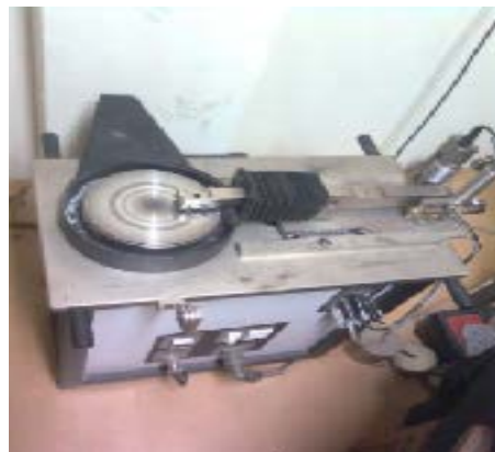
Figure 2.3 Pin –on-Disc wear testing machine
