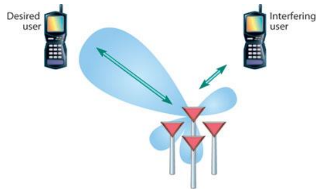
Fig.1. Basic diagram of smart antenna
