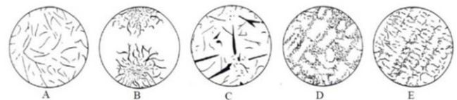
Fig. 1 Reference images for the five classes of graphite particles according to standard EDS-T-7101
