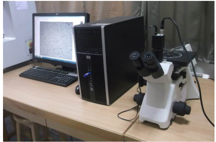
Fig. 3 Microscopic setup with CCD camera and attached computer
