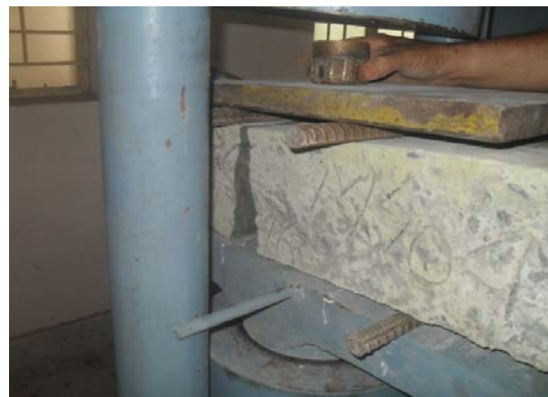
Photo 6- Failure of concrete beam
