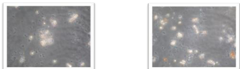
Phase contrast microscopic pictures identify microorganisms and white calcium carbonate crystals formation
