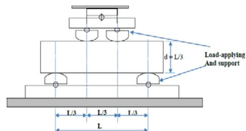
**Fig 3.2 Diagrammatic view of flexure test of concrete by third-point loading Method**
