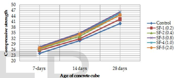
**GRAPH 4.1 COMPRESSIVE STRENGTH AT 7, 14 AND 28 - DAYS OF AGE AT 0%, 0.2%, 0.4%, 0.8%, 1% AND 2% OF STEEL FIBER TO THE OPTIMUM PERCENTAGE OF SILICA FUME.**
