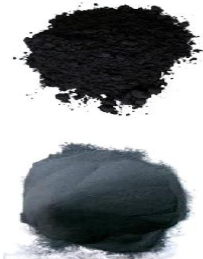
Fig.1.2. Silicon Carbide and Graphite Particulates
