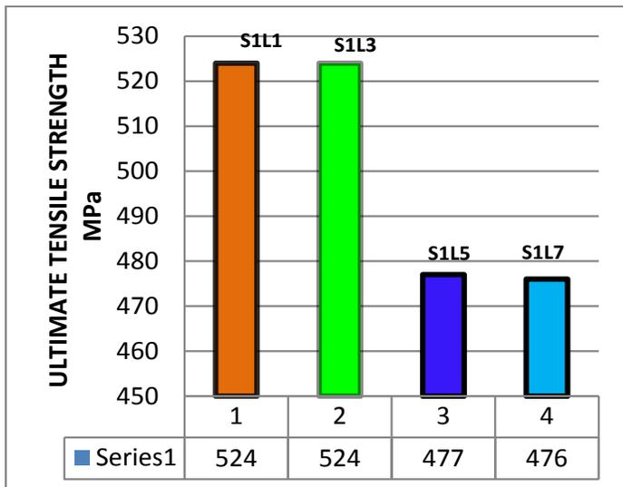
Fig.22. Ultimate tensile strength of different heat treatment Sample S1L1, S1L3, S1L5 and S1L7
