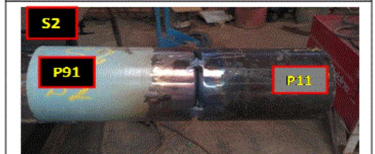
Fig. 1 Weld joint between P91 and P11 Pipe (a) Sample 1 (b) Sample 2
