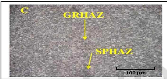
Fig.14c SPHAZ and FGHAZ 2 hours
