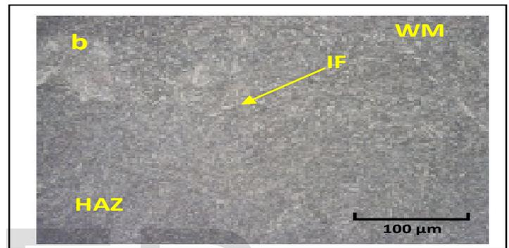
Fig. 9b Interface of P91 with weld metal
