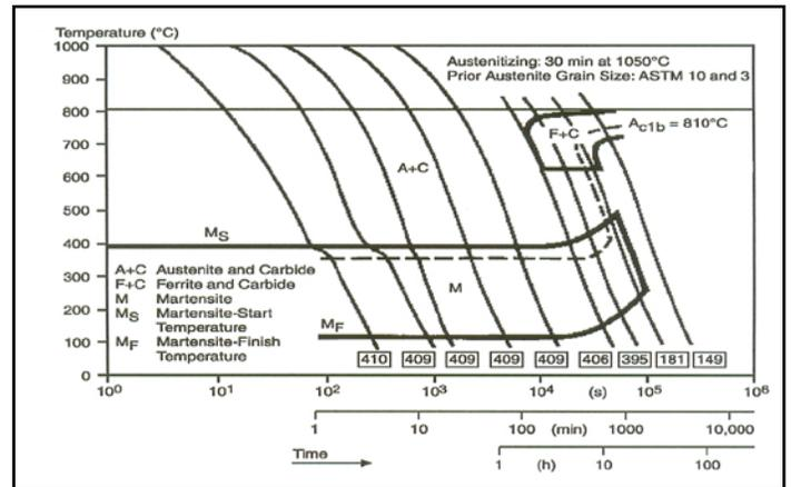
Figure 6 CCT diagram of steel P91[6].
