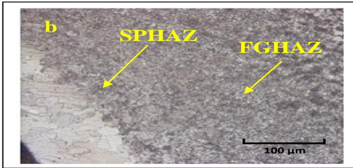
Fig.14b SPHAZ and FGHAZ 1 hour
