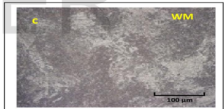
Fig. 9c weld metal of P91
