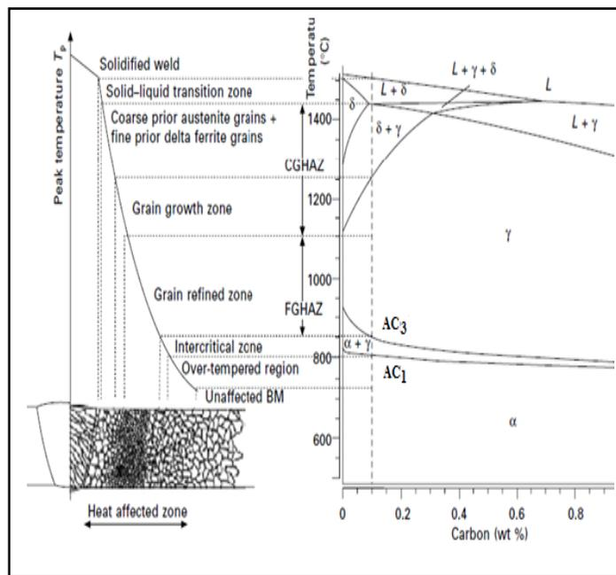
Figure 5 Schematic representations of microstructures developed in weld metal and HAZ as function of peak temperature
