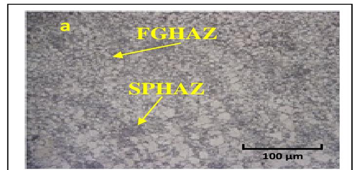
Fig.14a SPHAZ and FGHAZ 0.5 hour
