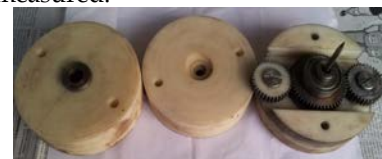
Figure 1 CFAAFM fixture parts and rotating attachment
