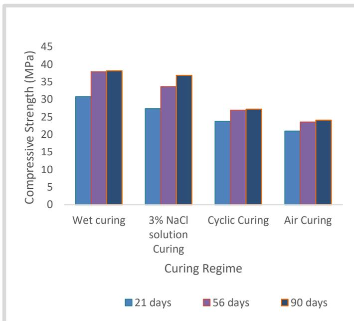
Figure.4 Average Compressive strength Comparison
