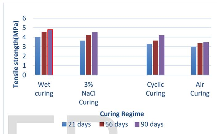
Figure.6 Average Flexural strength Comparison
