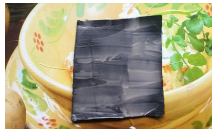
Figure 13: Sample 03 Silicone - 5.0g Acrylic Matt Topcoat - 5.0g
