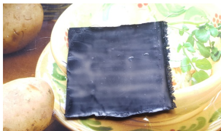
Figure 10: Sample 01 Silicone - 3.5g Acrylic matt Topcoat - 5.0g
