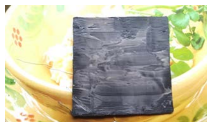
Figure 12: Sample 04 Silicone - 8.0g Acrylic Matt Topcoat - 5.0g
