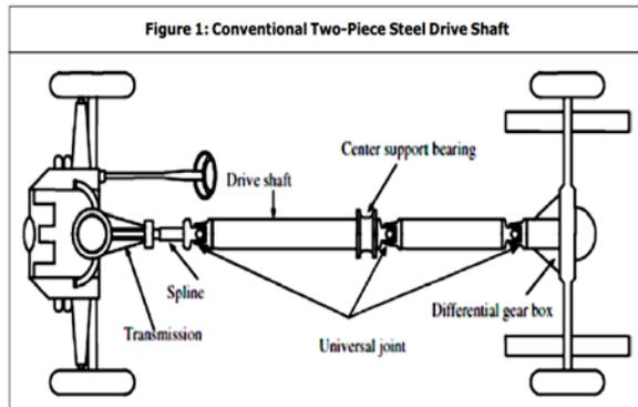
**Fig:1 Conventional two piece steel drive shaft**
