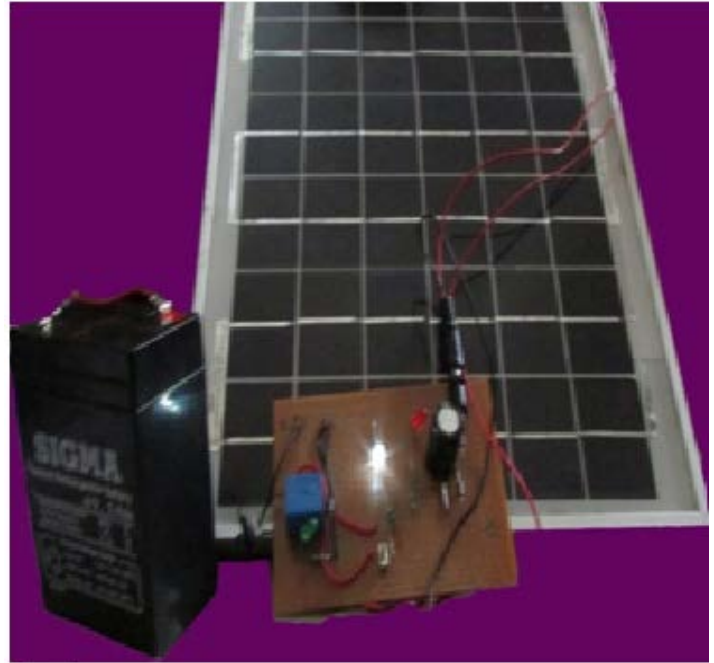
CaseII: Load is connected with the battery when solar energy is unavailable.
