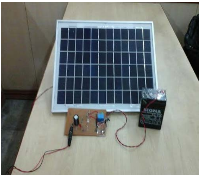
CaseI: Battery is getting charged from Solar energy and load is disconnected.
