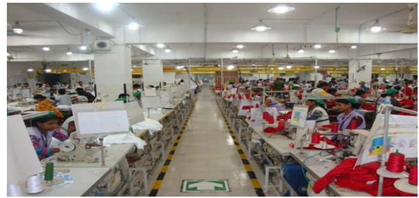
Figure3: Progressive Bundle System (PBS) [20].
