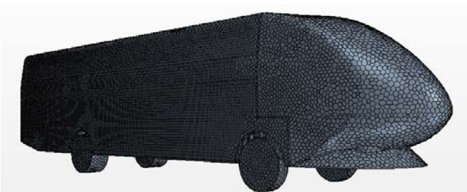
Fig. 3. Bus 4 with unstructured polyhedral mesh
