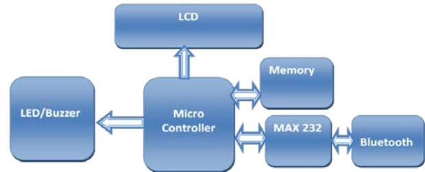
Fig. 2. Block diagram of Host
