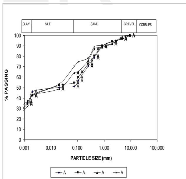
Fig. 4. Grading curves of soils from pit A
