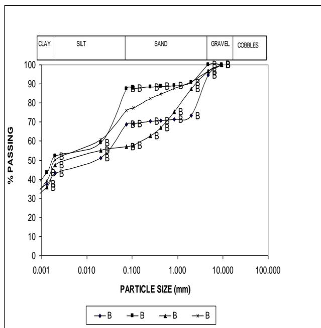
Fig. 5. Grading curves of soils from pit B
