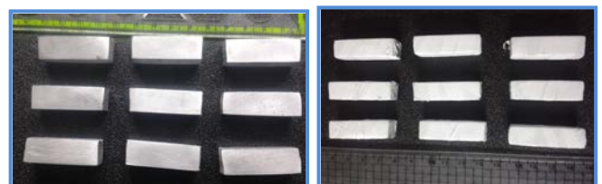
Fig.4 The samples before ECAP where they are warped by Teflon
