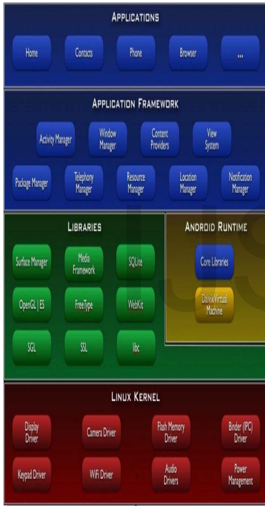
Figure 2.1: Android Operating system layers
