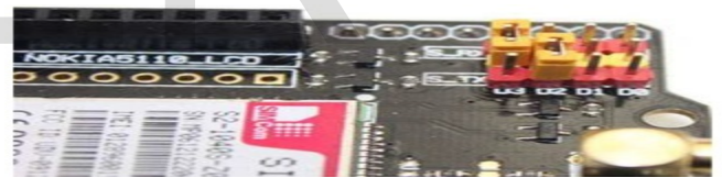
Fig. 10 LCD5100 interface and serial port
