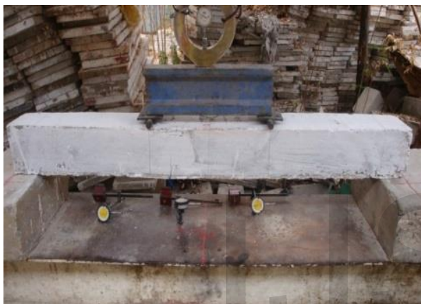
Plate. 3. Two Point Load Arrangement
