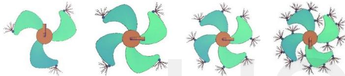
Fig. 3, a, b. One nozzle at each blade, c. Two nozzles, d. four nozzles
