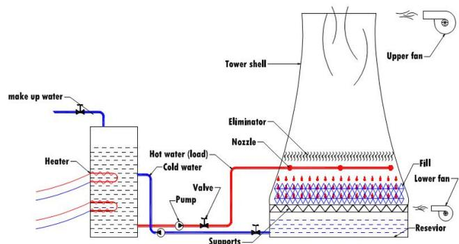
Fig.1 Schematic diagram for experimental test rig [4, and 5].
