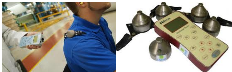
Figure 3: wireless110A Personal Noise Dosimeter and Data Collection approach
