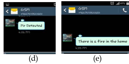
Fig.15. Receiving message alarm from AM-side: (a) Screenshot of MP-side at instance of receiving temperature alarm SMS. (b) Screenshot of MP-side at instance of receiving humidity alarm SMS. (c) Screenshot of MP-side at instance of receiving Gas alarm SMS. (d) Screenshot of MP-side at instance of receiving motion alarm SMS. (e) Screenshot of MP-side at instance of receiving Flame alarm SMS.
