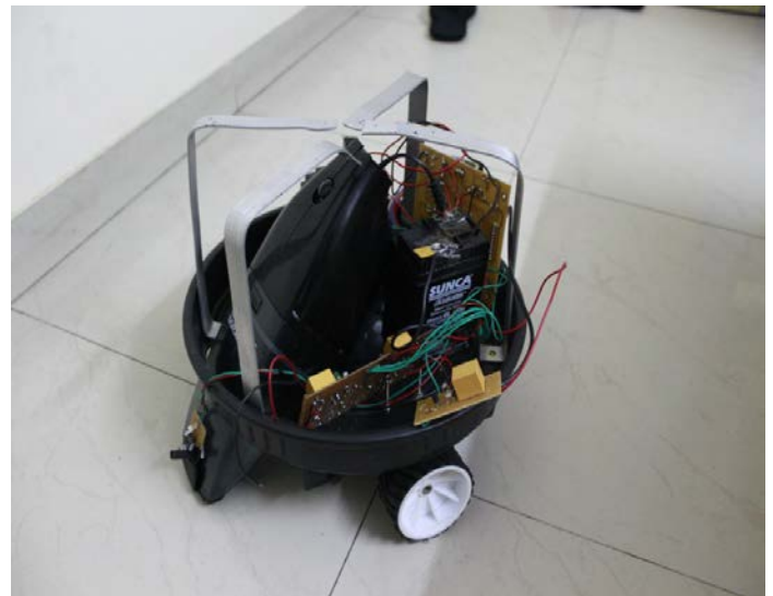
Figure 5: Shows the finished project. Entire system is functioning accordingly. The sensors can detect the obstacle. The 89S51 also can control the output device correctly like vacuum and switching Robot to Manual control.
