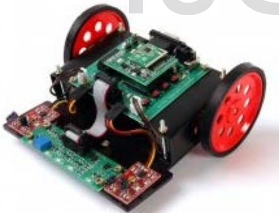
Fig. 1: A basic line following robot (Prototype of driving unit)
