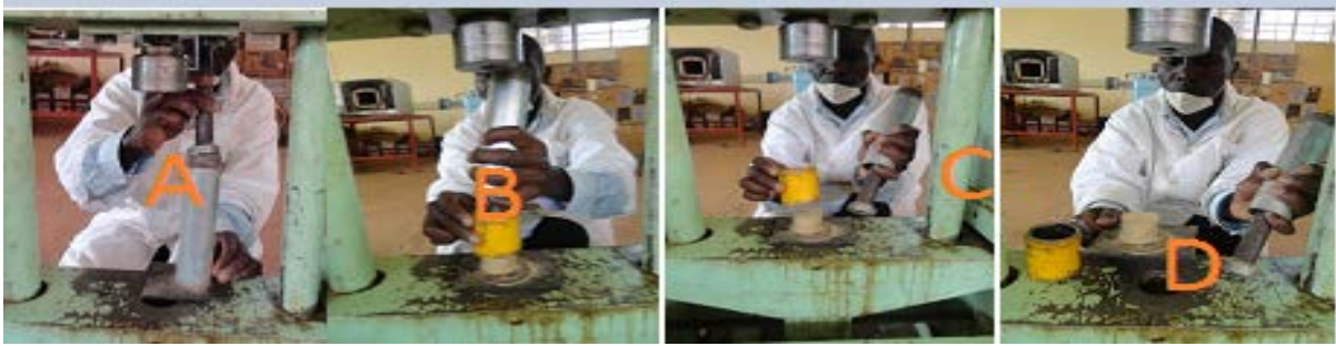
Plate 1: Briquetting process (A-Directing the piston; B, C &D- extruding briquette from the die)
