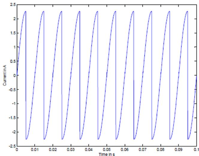
Figure 14: Output Current waveform for 100 Hz
