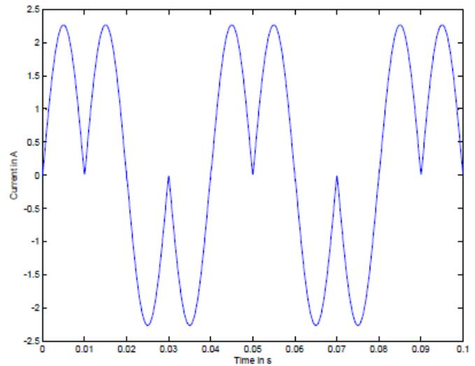
Figure 10: Output Current waveform for 25 Hz
