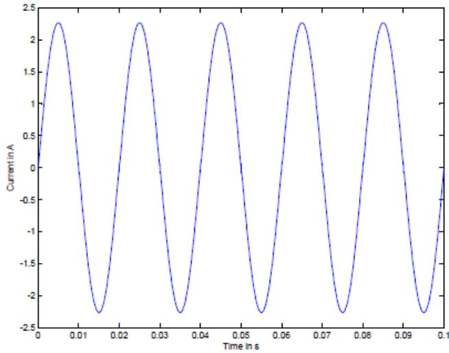
Figure 12: Output Current waveform for 50 Hz
